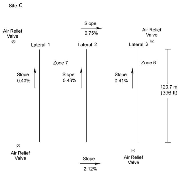
Figure 3. Orientation of drip laterals at site C.
