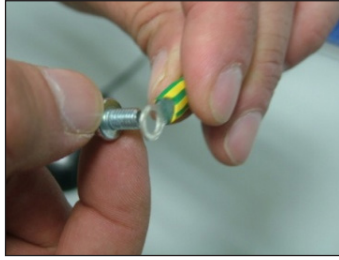
STEP 1 Insert the M5 screw through the pre-assembled Ring Terminal Lug.
