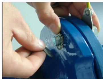
STEP 8 Add the flat washer on top of the serrated washer.
